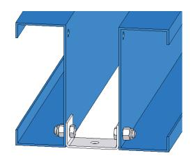
Assemble the frame. (4 screws CHC M8 x 20 + washer + nuts H)
