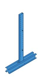
Screw on the fixing plates. (2 screws H M12 x 20 + locknuts)
